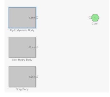
A variant sub-system is Simulink block type that allows the same toplevel model to follow several different execution pathways depending on the definition of a particular variable.
