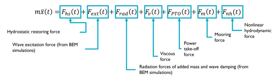
Excitation and radiation forces are determined from hydrodynamic coefficients calculated from Boundary Element Method (BEM)
