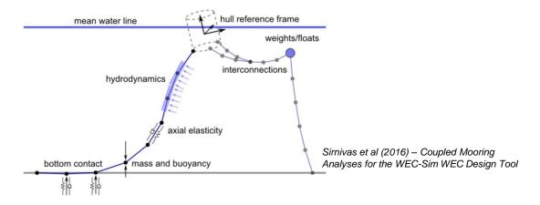
Dynamic mooring models are critical in order to obtain a more accurate estimate of a WEC's response and the mooring line loads.
