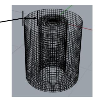
Some geometries require multiple embedded loops of panels i.e. top view:
